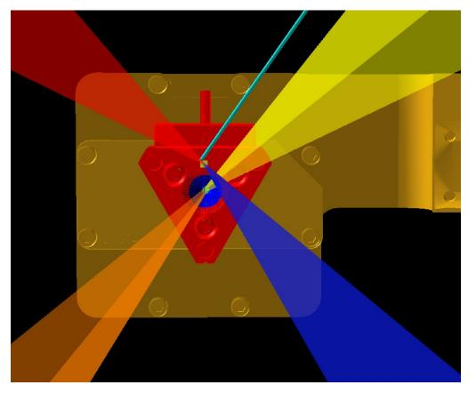
modified PXRDIP with new front plate design to hold DAC target
